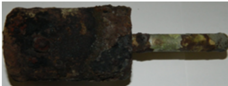
Figure 19 Cylinder electroplated in lab: After 20 cycles
