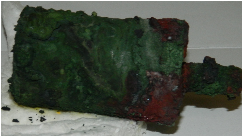
Figure 41 Chrome-plated cylinder (150 \mu\text{m} ) failed after 3 thermal cycles
