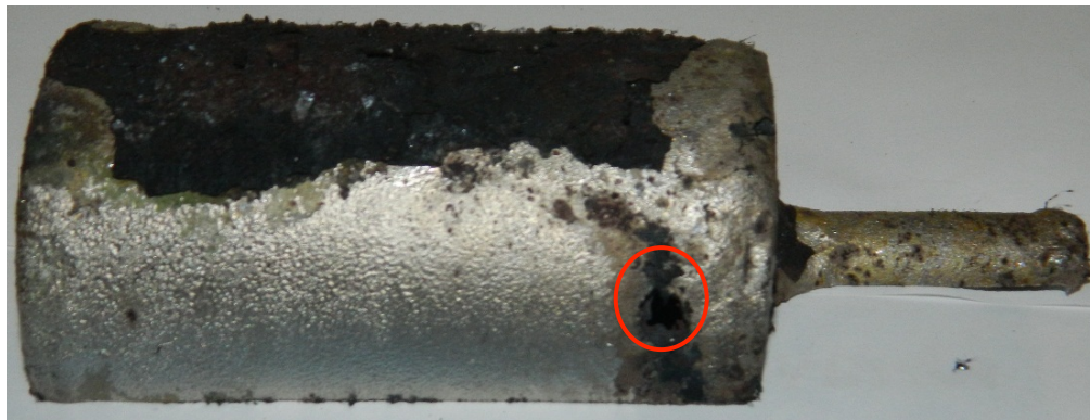
Figure 34 Electroplated Ni cylinder A (150 \mu\text{m} of electroplated nickel) after 200 cycles and the point of failure
