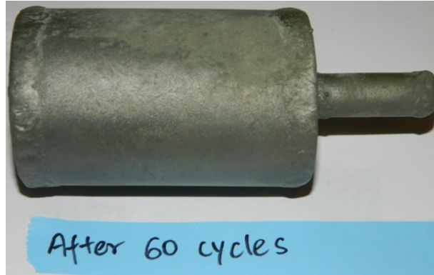
Figure 33 Electroplated Ni cylinder A (150 \mu\text{m} of electroplated nickel) after 60 cycles
