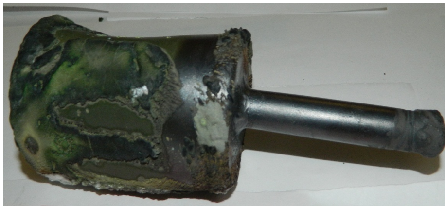
Figure 31 Failure of electroplated 150 \mu\text{m} Ni cylinder between 1700 and 1800 cycles
