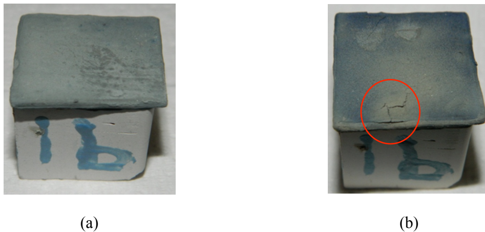
Figure 3 Sealmet sample: (a) Before testing; (b) After testing: cracks observed
