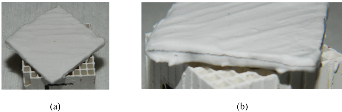
Figure 7 Alumina adhesive + silica: (a) Before testing; (b) After testing: crack
